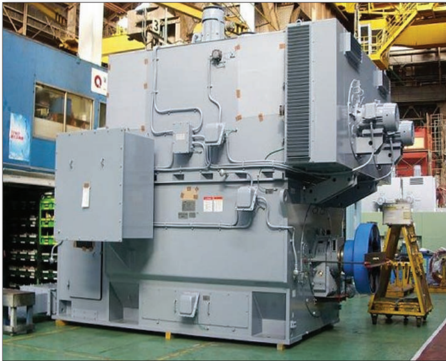
Figure 2: This TMEIC 6,500 HP TEAAC motor operates as part of a liquids pipeline in the U.S.
