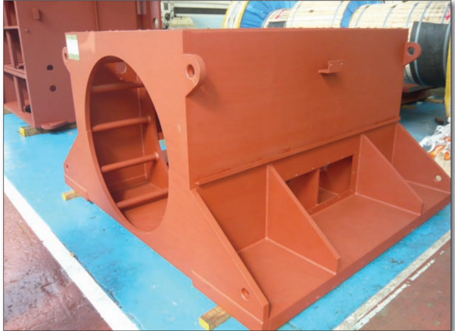
Figure 1: Bare frame before the winding is installed
